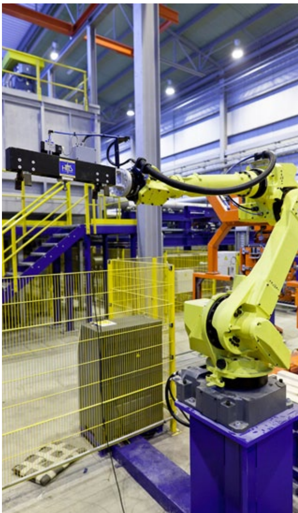
A robot handles the wood used for stacking of billets.
